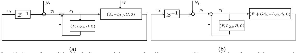
Fig. 5. (a) A transform of the block diagram of the general coding structure. (b) An equivalent form of the communication system driven by GM inputs.
