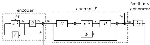
Fig. 3. A general coding structure for  $\mathcal{F}$ .
